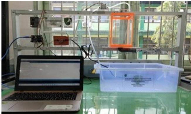
Gambar 6. Prototype sistem kendali level cairan.
