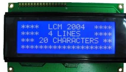
Gambar 7. Liquid Crystal Display (LCD) 20x4
