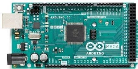
Gambar 3. Arduino Mega 2560
