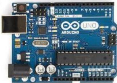
Gambar 3. Board Arduino Uno [15].
