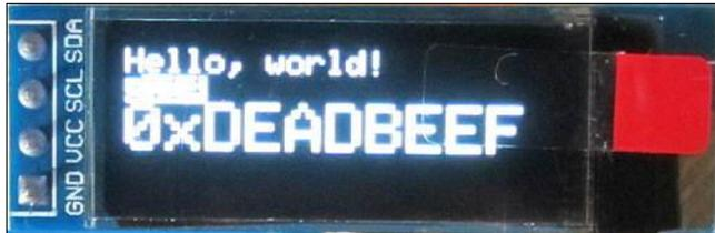
Gambar 4. LCD Oled 128x32 [7]
