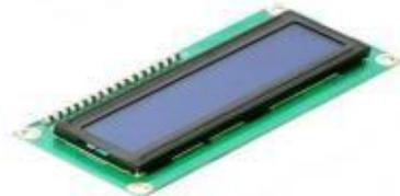
Gambar 10. Liquid crystal display (LCD) [10]
