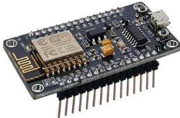
Gambar 6. NodeMCU ESP8266 [8]
