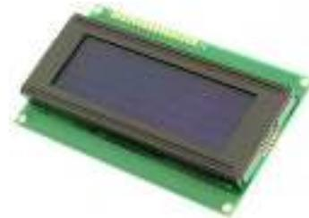
Gambar 4. LCD 20x4
