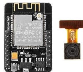
Gambar 8. ESP32-CAM
