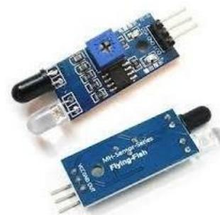
Gambar 7. Sensor jarak infra red (IR)
