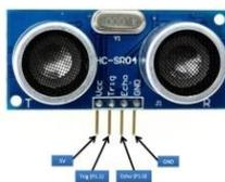
Gambar 4. Sensor ultrasonik HC-SR04 [12]
